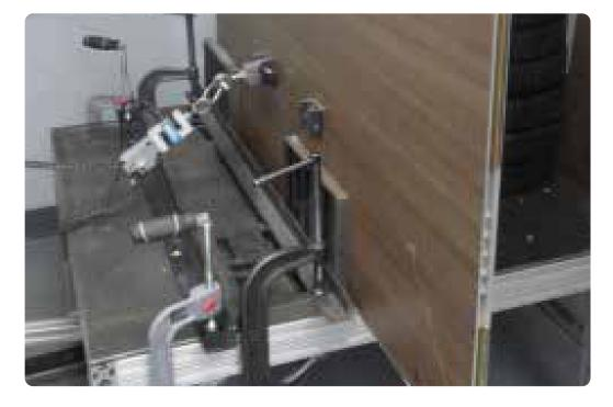
A Bond Test demonstrated the strength of the bond between the panel and frame.
