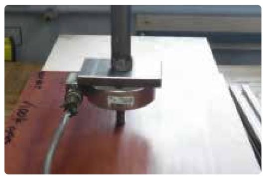
A Puncture Test demonstrated the floor can withstand 500-lbs of pressure from a stiletto heel.
