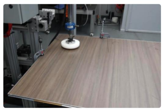
The Load Cycling Test showed the floor can withstand high impact in the same location of up to 500 lbs of weight without sustaining damage.
