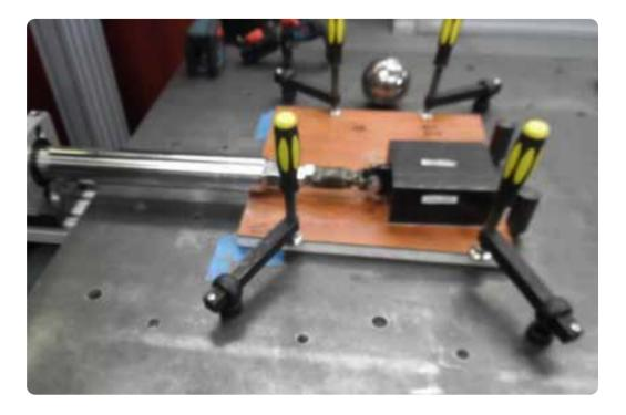
A Scratch Abrasion Test showed the surface will not scratch when dragged over rough carpet or concrete flooring.
